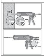
Inject the mortar from the back of the hole towards the front and slowly withdraw the mixing nozzle step by step after each trigger pull.
