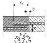
Critical temperature-dependent bond stress,  $\tau_c$ , concerning "overlap joint" for Hilti HIT-RE 500-SD injection adhesive in relation to fire resistance class and required minimum concrete coverage c.
