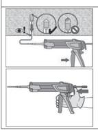
Insert piston plug to back of the hole. Begin injection allowing the pressure of the injected adhesive mortar to push the piston plug towards the front of the hole.
