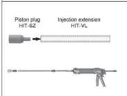
Assemble mixing nozzle HIT-RE-M, extension(s) and piston plug HIT-S7
