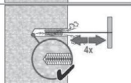
Brush 4 times with the specified brush size by inserting the steel brush Hilti HIT-RB to the back of the hole (if needed with extension) in a twisting motion and removing it. The brush must produce natural resistance as it enters the bore hole -- if not the brush is too small and must be replaced with the proper brush diameter.
