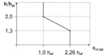
For spacing (or edge distance) smaller than critical spacing (or critical edge distance) the design loads have to be reduced.
