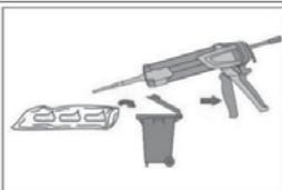
Discard initial adhesive. The foil pack opens automatically as dispensing is initiated. Depending on the size of the foil pack an initial amount of adhesive has to be discarded.
