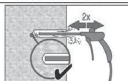
Blow 2 times from the back of the hole (if needed with nozzle extension) over the hole length with oil-free compressed air (min. 6 bar at 6 m<sup>3</sup>/h) until return air stream is free of noticeable dust.
