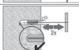
Brush 2 times with the specified brush size by inserting the steel brush Hilti HIT-RB to the back of the hole (if needed with extension) in a twisting motion and removing it. The brush must produce natural resistance as it enters the bore hole -- if not the brush is too small and must be replaced with the proper brush diameter.
