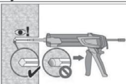
Inject the adhesive starting at the back of the hole, slowly withdrawing the mixer with each trigger pull. Fill holes approximately 2/3 full, or as required to ensure that the annular gap between the anchor and the concrete is completely filled with adhesive along the embedment length.
