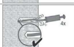
Blow out again with manual pump at least 4 times until return air stream is free of noticeable dust.
