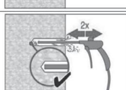
Blow again with compressed air 2 times until return air stream is free of noticeable dust.
