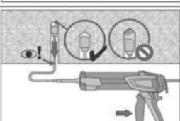
Overhead installation and/or installation with embedment depth  $h_{\text{ef}} > 250\text{mm}$ . For overhead installation the injection is only possible with the aid of extensions and piston plugs. Assemble HIT-RE-M mixer, extension(s) and appropriately sized piston plug. Insert piston plug to back of the hole and inject adhesive. During injection the piston plug will be naturally extruded out of the bore hole by the adhesive pressure.
