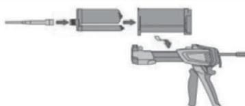
Tightly attach new Hilti mixing nozzle HIT-RE-M to foil pack manifold (snug fit). Do not modify the mixing nozzle. Observe the instruction for use of the dispenser. Check foil pack holder for proper function. Do not use damaged foil packs / holders. Swing foil pack holder with foil pack into HIT-dispenser.
