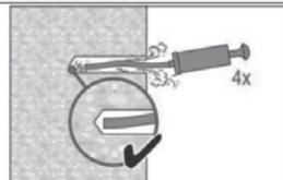
The Hilti manual pump may be used for blowing out bore holes up to diameters  $d_0 \leq 20\text{ mm}$  and embedment depths up to  $h_{ef} \leq 10\text{d}$ . Blow out at least 4 times from the back of the bore hole until return air stream is free of noticeable dust
