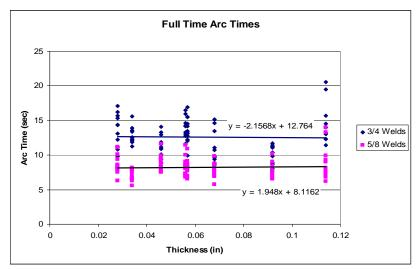
Figure 3-1: Arc Times for full-time Welds
