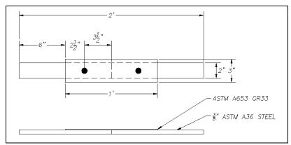
Figure 2-1: Test Specimen Configuration
