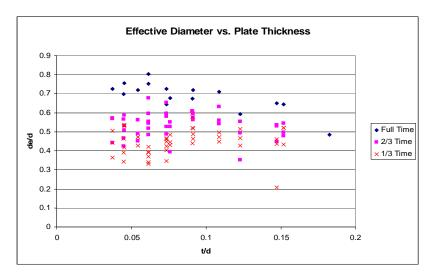
Figure 3-2: Measured Effective Weld Diameters
