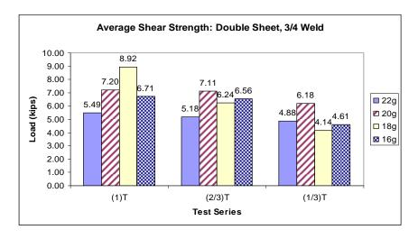
Figure 3-8: Average Shear Strength of 3/4 in. Welds in Double Sheets
