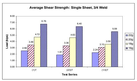
Figure 3-6: Average Shear Strength of 3/4 in. Welds in Single Sheets
