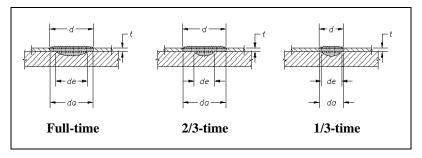
Figure 3-3: Common Weld Cross Sections
