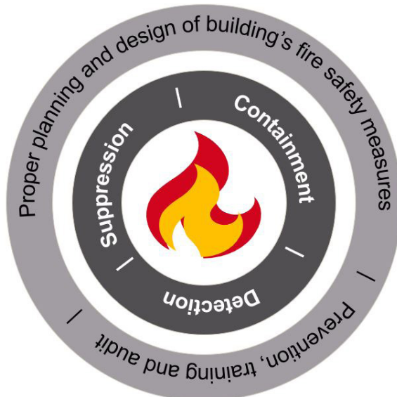
Figure 1.5 Elements of fire protection
