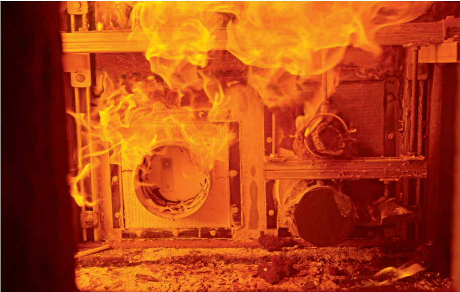
(c) Fire exposed side during the fire endurance test
